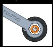
The spring preload is fundamental for the function of the suspension. If the preload is incorrectly set, any other adjustments will not help to get the intended performance from the suspension.
