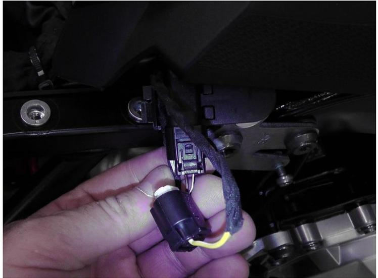
Take the new set out of the box and connect the EPA P&P Module.
