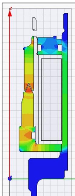
Countless calculations have been performed before the first prototype of the Tractive DDA valve was put to the test. The aim was high, the fastest and most stable bi – directional, internal proportional, damping valve with the utmost linear adjustment behavior. A valve that wouldn't be impressed by working temperatures below minus 30 degrees Centigrade or above 140 degrees Centigrade.
